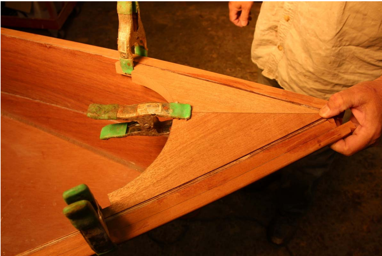
Spring clamps hold the breasthook while you take note of any necessary adjustments. (Note that the outwales have already been installed. It would be smart to have the Skerry's stock plywood breasthooks wedged in place temporarily during hull assembly to ensure that your bow and stern are shaped correctly.)
