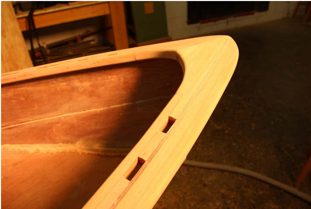
The round-over we gave the inwales was continued around the inside perimeter of the breasthook.
