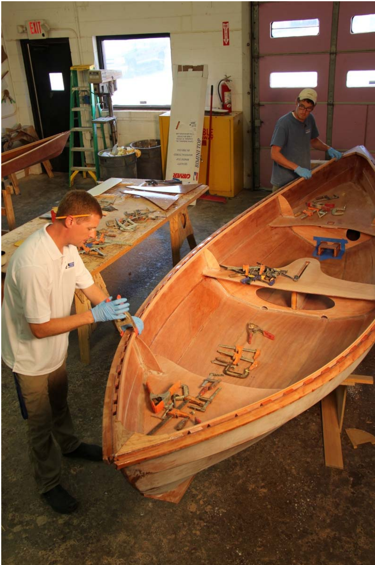
Minimizing the glue mess is essential here. Start with a couple of spring clamps to settle the inwale in place. Note C-clamps staged and ready.
