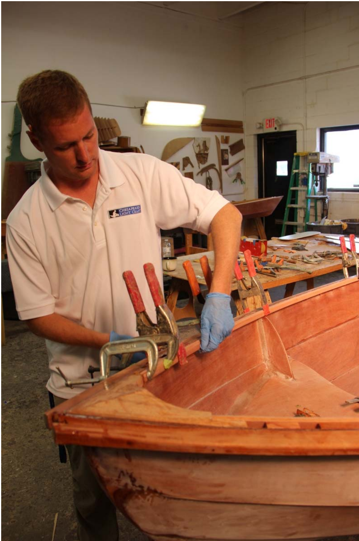
Watch the alignment! Don't want to glue the inwale in too high or too low in the boat.
