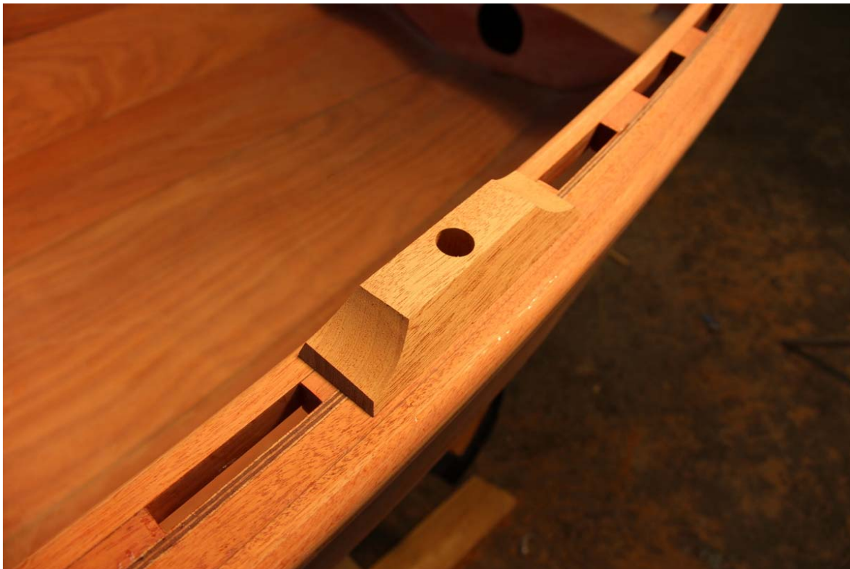
...And tested the fit on the boat. The carefully-designed angles in the sides of the mounting blocks position the oarlock socket so that the hole for the oarlock pin passes inboard of the plywood hull side.
