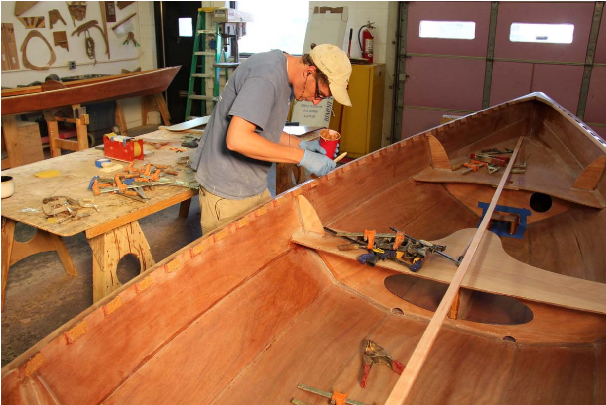
Out comes the glue, dabbed on the spacer blocks.
