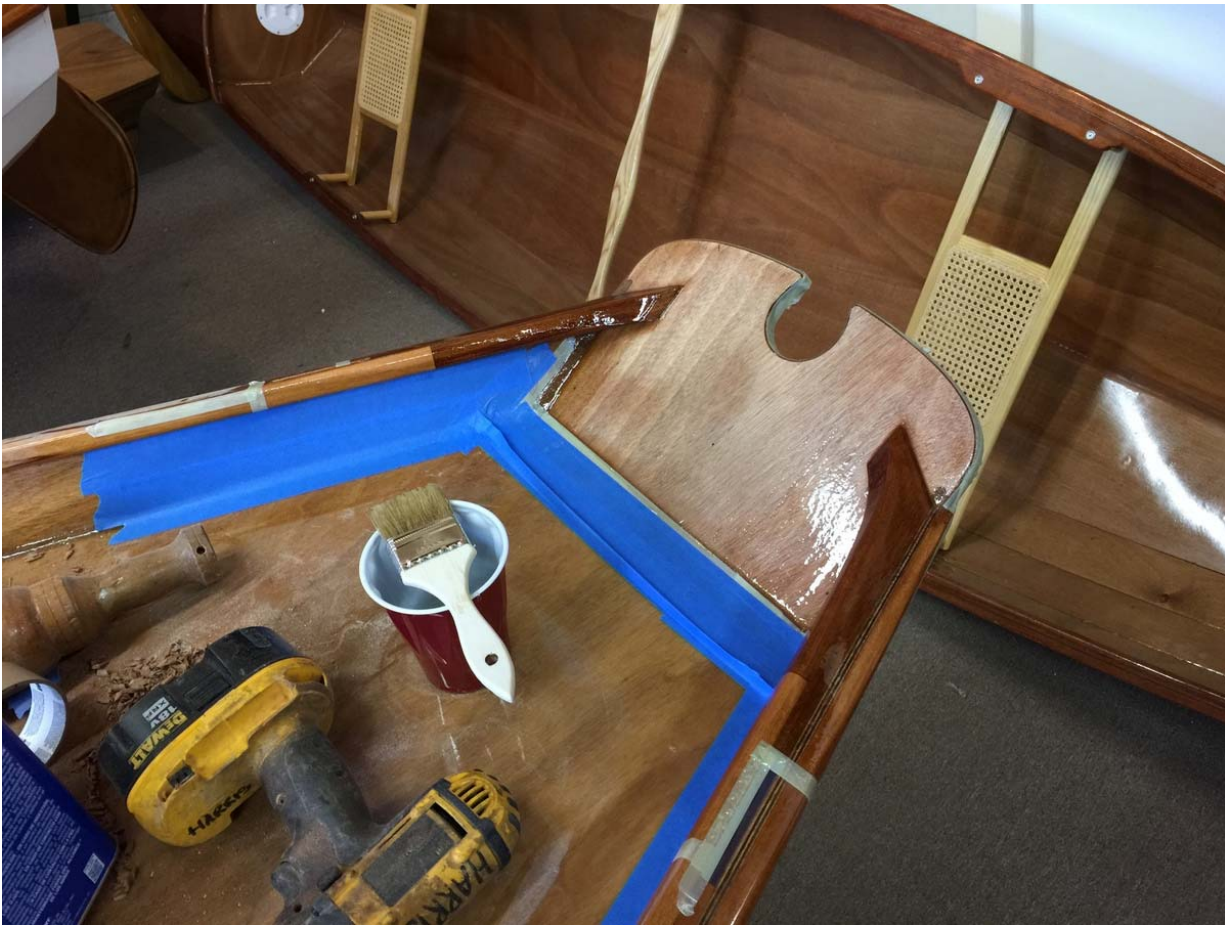
Here are the quarter knees on a Southwester Dory , fitted with the optional spaced inwales.
