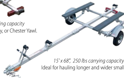
Single Light Duty Carrier Kit SUT-250-SCLCT
