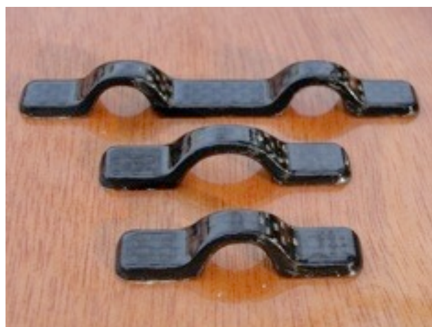
Glued and finished eye straps.
